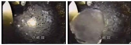
Fig.10 Dynamic behavior of liquid hydrogen, visualized during the pressurization in the extended engineering experiment [9] .
