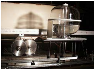
Fig.3 Electrical exciter for sloshing test.
